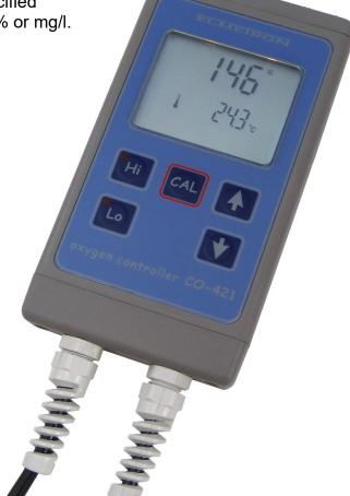
The meter enables storing of 8000 results. The built-in memory allows you to remember the results with a set time interval: the shortest 1 minute, and the next possibilities : 2, 5, 10, 15, 30, 60 minutes. When the memory is full, the oldest result is deleted and a new one is added. The results can be transferred to a computer via USB. The delivered in the set computer software allows to transfer the results of the measured function and temperature with the date and time of recording.
